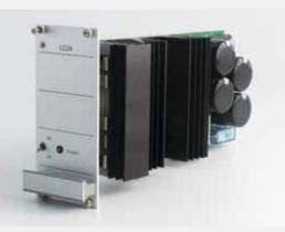
■ Figure 7.12: LC24A AC/DC converters for magnetic actuators
