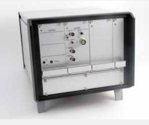
■ Figure 7.9: View of the SA75D switching power rack
