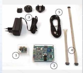
■ Figure 9.6: Components of the LSPA30uXS developer kit
