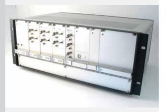
■ Figure 7.2: Customised rack including 6 channels & 3 closed loops
