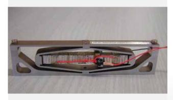
■ Figure 4.2a : Single blade guided Amplified Piezoelectric Actuator APA®
