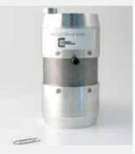
■ Figure 3.23: MICA200 Moving Iron Controllable Actuator
