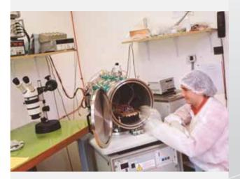
■ Figure 3.28b: View of CEDRAT TECHNOLOGIES labs, thermal Vacuum chamber
