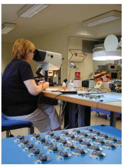
■ Figure 3.29a: Integration of a batch of piezoelectric mechanisms
