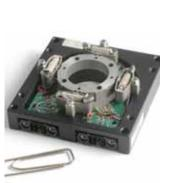
■ Figure 3.7a: XY stage based on APA25XS used for micro-scanning
