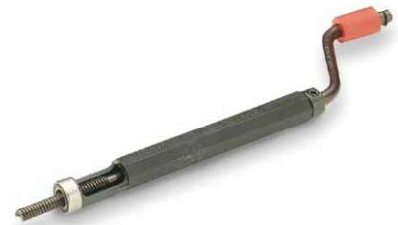
TYPE II Prewinder Prewinder reduces the diameter of the insert to that of the tapped hole allowing for easy installation.
